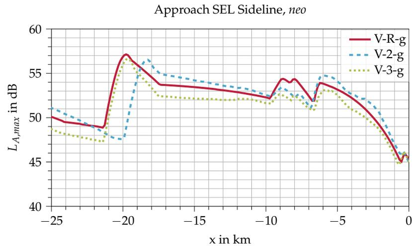
Figure 13.  $L_{A,max}$  level 1000 m sideline during approach (*neo*).
