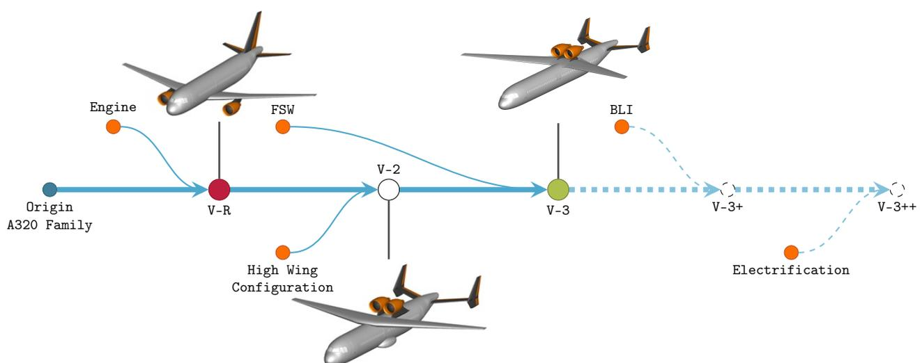
**Figure 4.** Evolution of low noise aircraft design at DLR.
