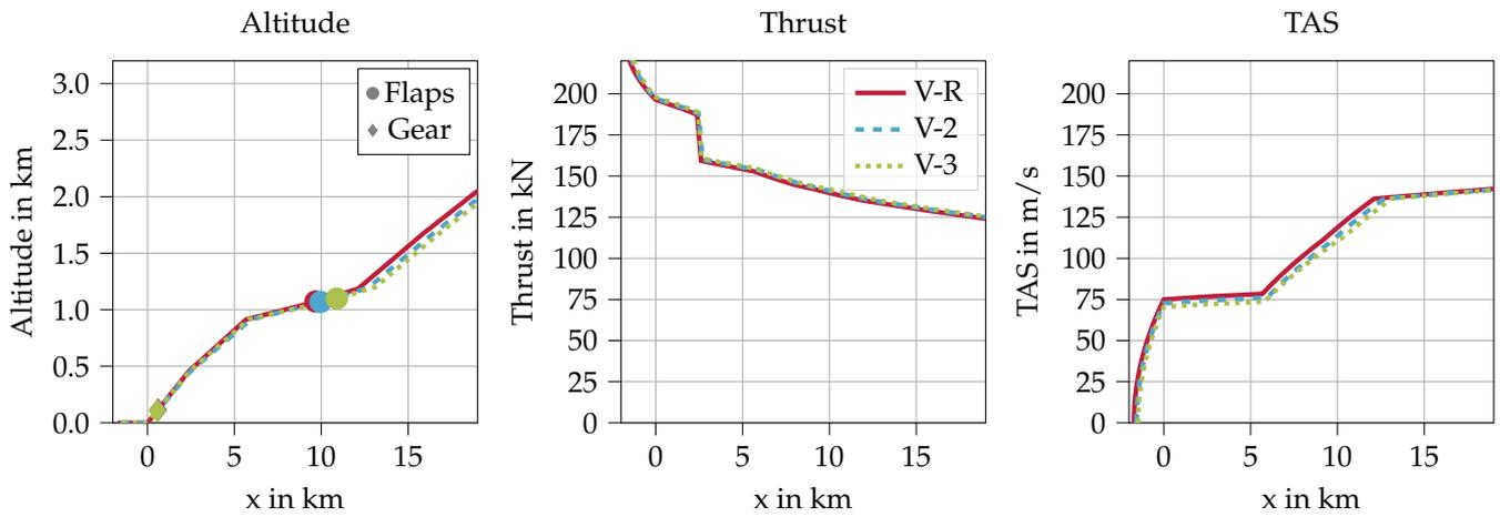
Figure 8. Departure trajectories: current engine option (BPR = 6).
