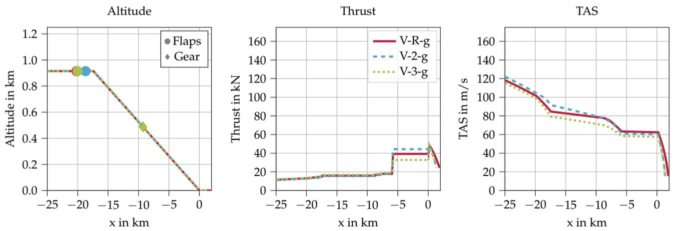
Figure 9. Approach trajectories: new engine option (BPR = 12).
