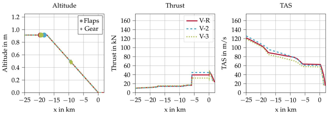
**Figure 7.** Approach trajectories: current engine option (BPR = 6).
