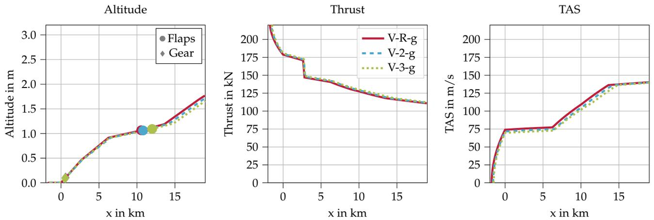
Figure 10. Departure trajectories: new engine option (BPR = 12).
